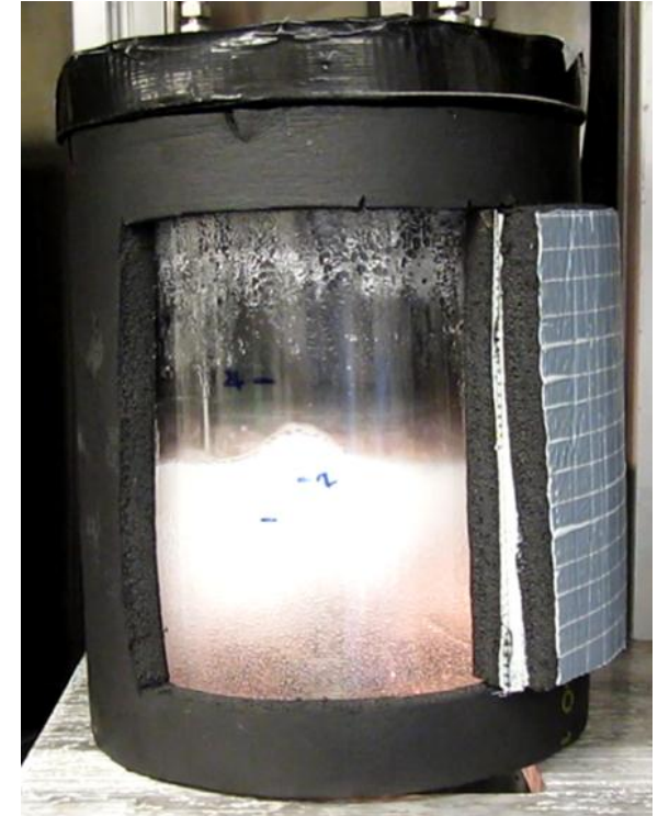
Loaded Solvent at 70°C – With Sonication
